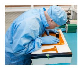
Each of the fingers is individually inspected to ensure that the there are no defects in the plating layer that could outgas at a later stage.
